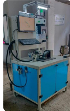
POKA YOKE AND QR CODE PRINTING STATION FOR ELBOW TYPE OF PART
