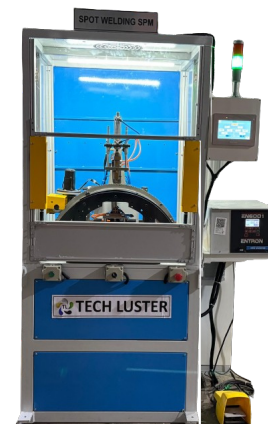
SPOT WELDING SPM AUTOMATION FOR AEROSPACE COMPONENTS
