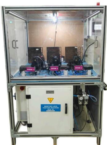
PROGRAMMABLE LIFECYCLE TESTING OF MORTISE LOCK - DOOR LATCH
