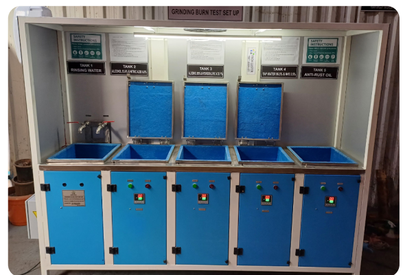
TBT 450L-7T DIGITAL TIMER BASED GRINDING BURN TEST SETUP
