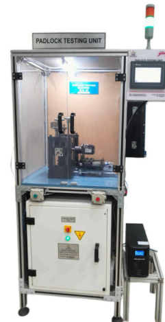
PROGRAMMABLE LIFECYCLE TESTING OF PADLOCK
