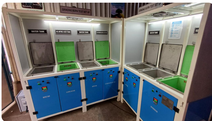
TBT 450L-7T DIGITAL TIMER BASED GRINDING BURN TEST SETUP
